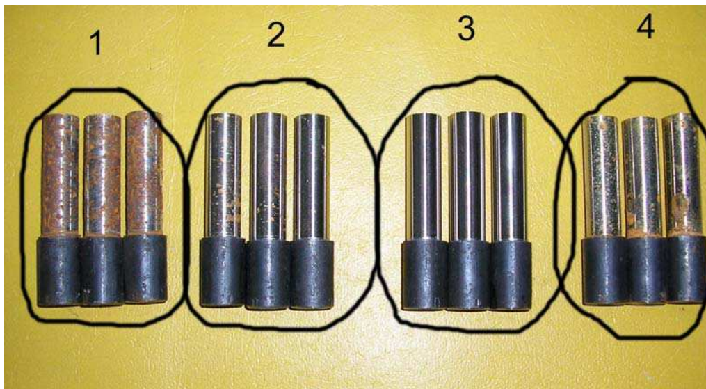
Figure 2. Appearance of samples machined without application of coolant (dry machining) after testing: 1-in salt chamber, 2-in atmospheric conditions, 3-in closed area, 4-in wet chamber.
