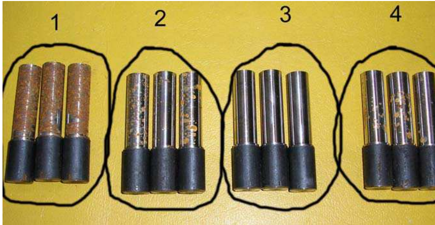
Figure 5. Appearance of samples machined with application of SHIP coolant containing inhibitor INH3 after testing 1-in salt chamber, 2-in atmospheric conditions, 3-in closed area, 4-in wet chamber
