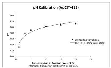
Please note the solutions used above were created using deionized water. Slight differences in water chemistry (dissolved solids, hardness, etc.) may lead to differences in readings. Please use these numbers as reference only; Contact Cortec® Laboratories with any questions.
