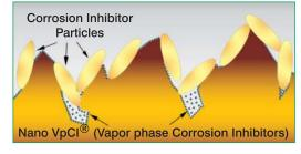
Cortec® Coatings are unique because the Nano VpCl® (Vapor phase Corrosion Inhibitors) penetrates and protects the micro-cavities against micro-corrosion.
