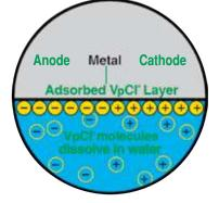
**VpCI** technology is a revolutionary, environmentally safe, and cost-effective option for corrosion protection. Cortec products protect with a thin, monomolecular protective film. The barrier re-heals and self-replenishes; and can combine with other functional properties for added protective capabilities.
